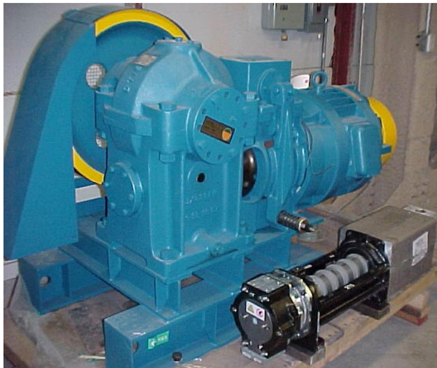
Gen2 Machine (foreground) Compared to a Traditional Traction Machine (background)
